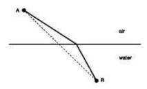
"This hypothetical path is shorter than the path the light actually takes. But light travels more slowly in water than it does in air, and a greater percentage of this path is underwater. So it would take longer for light to travel along this path than it does along the real path."
