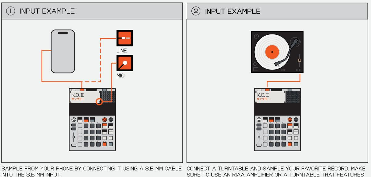
SURE TO USE AN RIAA AMPLIFIER OR A TURNTABLE THAT FEATURES A BUILT-IN AMP.
