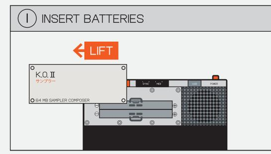
LIFT OFF THE TOP LID TO REVEAL THE BATTERY COMPARTMENT.
