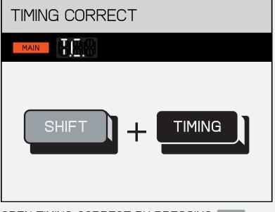
OPEN TIMING CORRECT BY PRESSING SHIFT AND TIMING .
