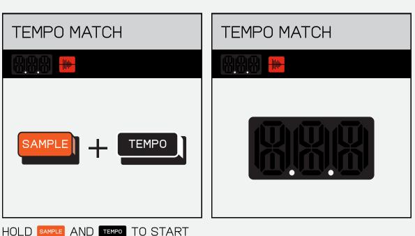
HOLD SAMPLE AND TEMPO TO START LISTENING FOR THE INCOMING AUDIO, THEN PLAY ANY AUDIO INTO THE DEVICE THROUGH THE LINE-IN OR INTO THE MIC. K.O. II WILL LISTEN, FIND THE TEMPO, DISPLAY IT ON SCREEN AND THEN SET THE PROJECT TEMPO TO MATCH.
