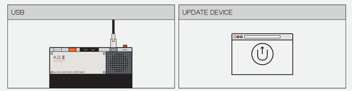
YOU CAN ALSO POWER THE UNIT WITH A STANDARD USB-C CABLE (5V / MIN IA). WE RECOMMEND USING A QUALITY 'USB-IF' COMPLIANT CABLE. KEEP YOUR K.O. II UP-TO-DATE WITH THE LATEST FIRMWARE BY GOING TO:
